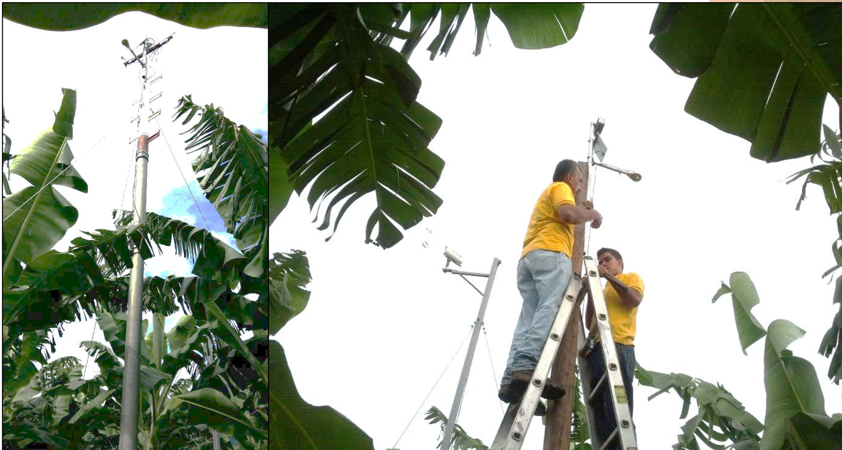
Installation of the weatherstation at crop height (WWF Mejia, 2012)
